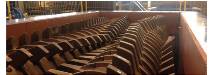
Sizer SWB0740, rotor diameter 700 mm, rotor width 4000 mm, coal 2500 t/h
