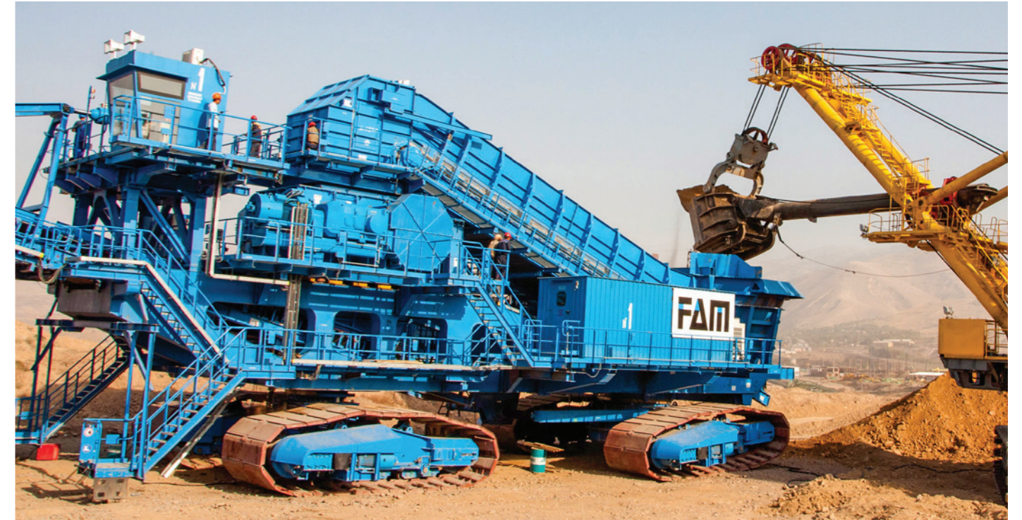
In-pit crushing system FZWB2025, on crawlers, double roller crusher ZWB2025, apron feeder AF2600x21, belt conveyor stationary GF2000x24, overburden 5250 t/h
