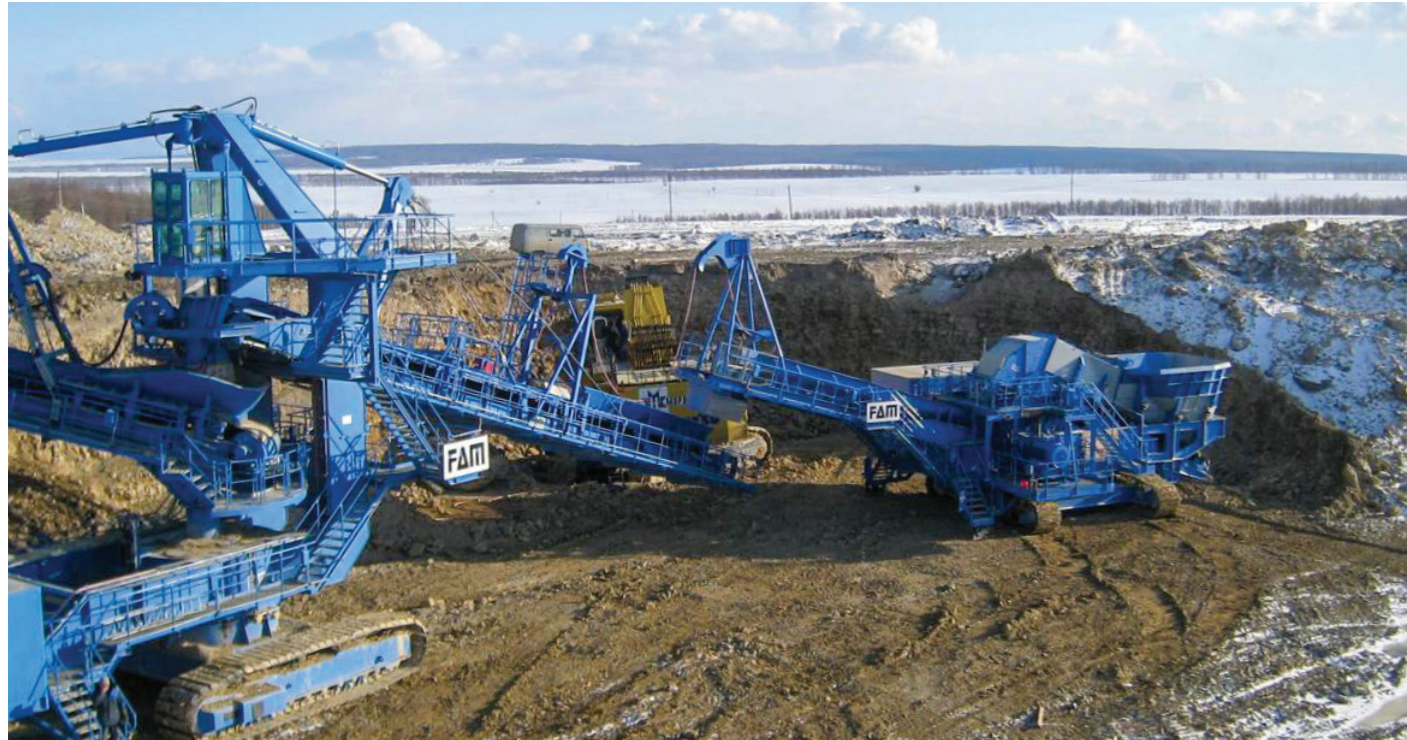
In-pit crushing system FPB1314-20/13.5, on crawlers, apron feeder AFs1600x8,5, impact crusher PB1314, belt conveyor stationary GF1600x13,9, overburden, chalk 1700 t/h
