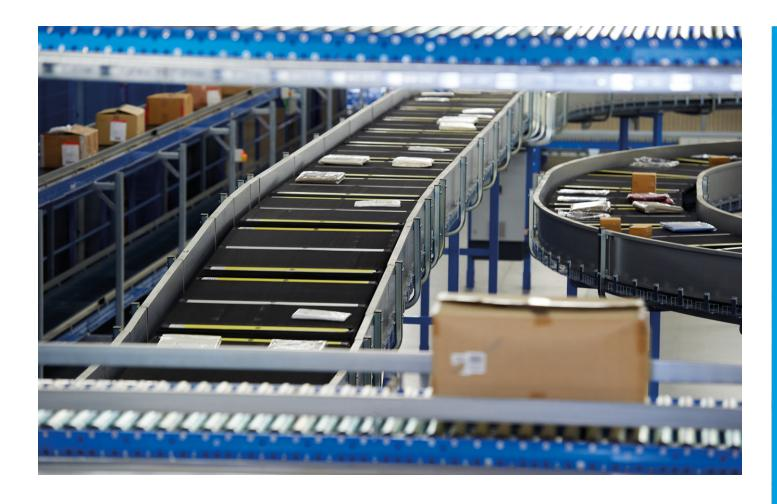
The use of a common sorter platform and frame adds to system modularity and longevity and enables extensions or upgrades to accommodate further increases in capacity, all while the software provides the ability to change sortation parameters to match future changes in business needs.
