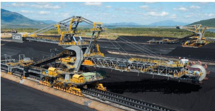
Stacker-reclaimer STR6000/8000.60, hard coal 8000 t/h, Australia
