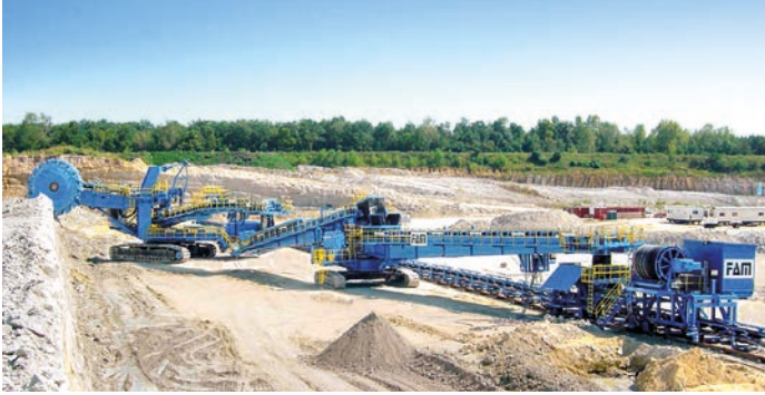
Transfer conveyor on crawlers BW1200.22/28R, bridging length 50 m, marl 2300 t/h, 1600 m 3 /h, USA
