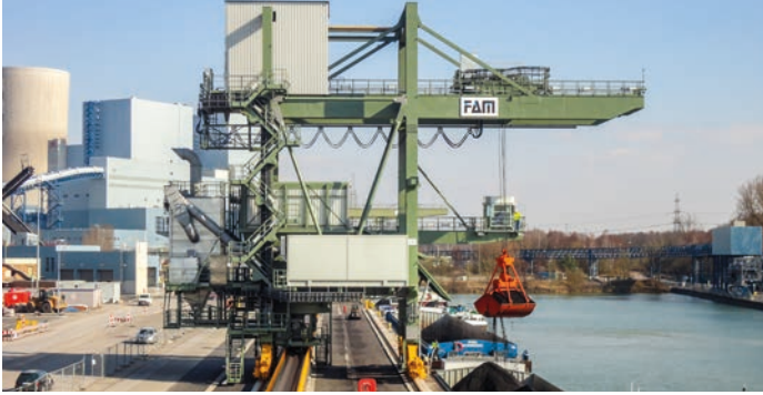
Ship unloader GUL1000.13KG, mobile, hard coal 1000 t/h, Germany
