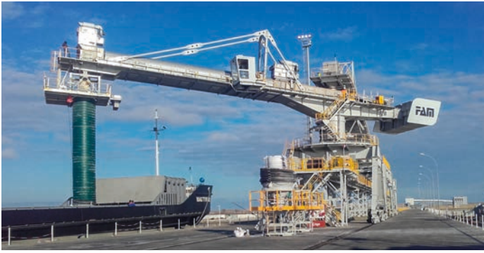
Shiploader SL1200.31.D.H, mobile, loading with cascade chute, urea 1200 t/h, Turkmenistan
