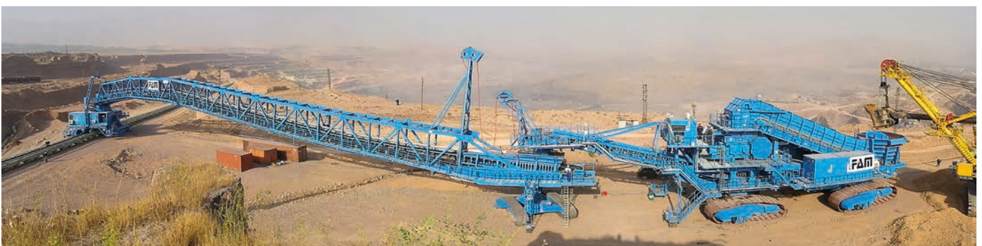
In-pit crushing system FZWB2025, on crawlers, overburden 5250 t/h, Uzbekistan
