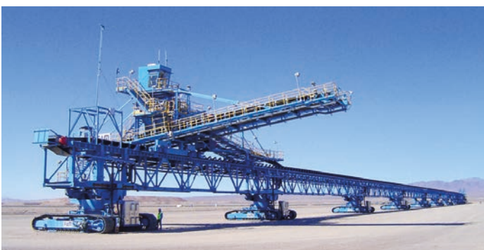
Conveyor bridge on crawlers MSB3480.9TC with tripper car, copper sulfide 3500 t/h, Chile
