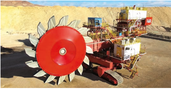
Bucket wheel excavator SR800P9, leached copper ore 9650 m 3 /h, 14500 t/h, Chile
