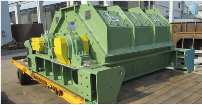
Double roller crusher ZWB0815MS-H, burnt lime 130 t/h, Germany
