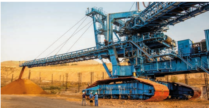
Spreader ST12100.60, overburden 12100 t/h, 8100 m 3 /h, Uzbekistan
