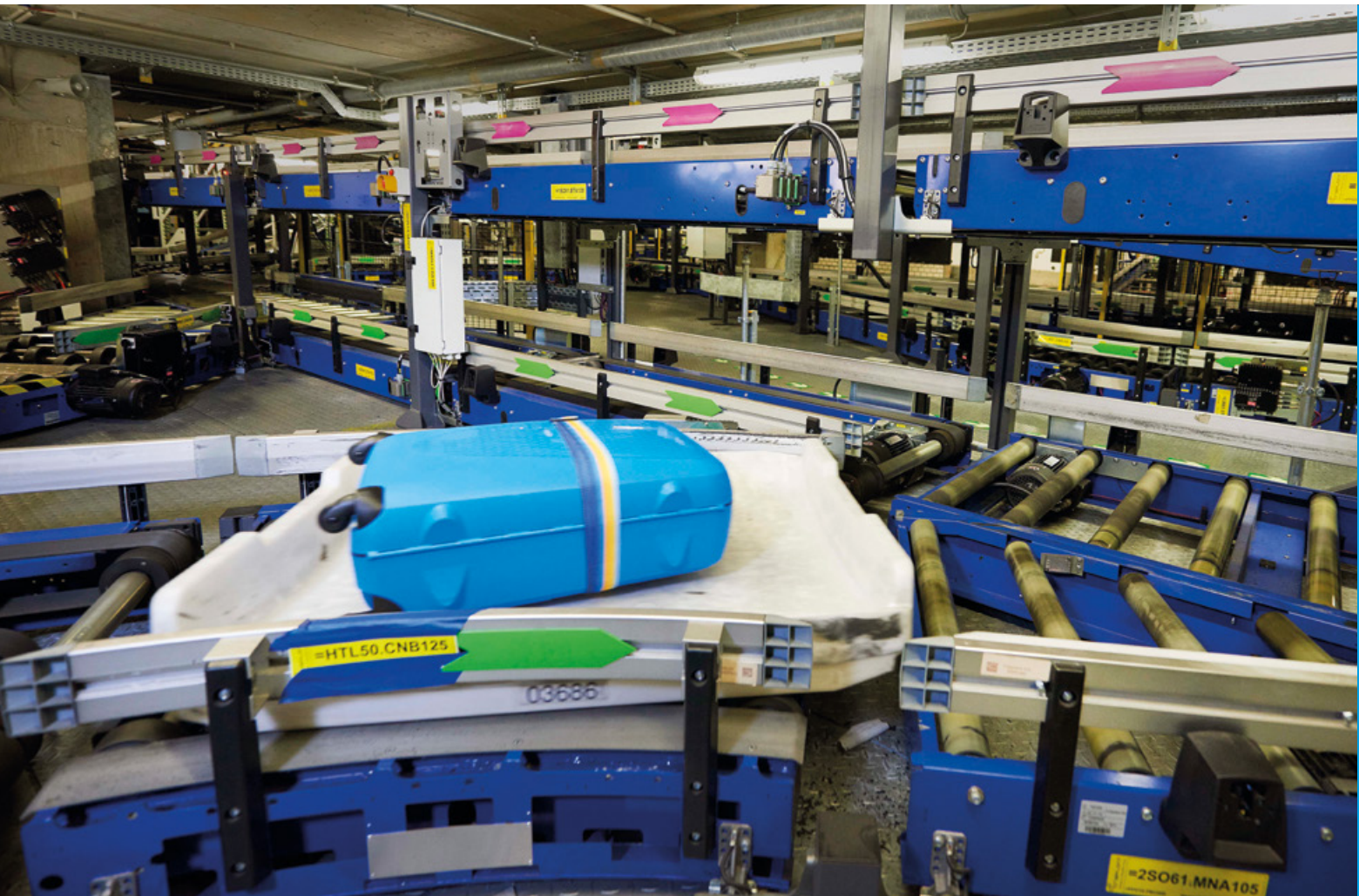
High speed baggage handling systems minimise baggage transfer times to speed up passenger flow and shorten connection times.
